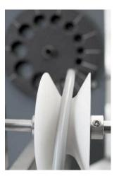
Automatic feeding of cables using the dereeling systems from ramatech
